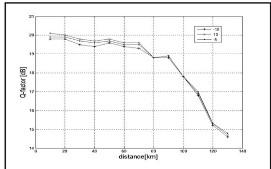
**Fig. 4: Transmission distance versus Q-factor for proposed system.**
