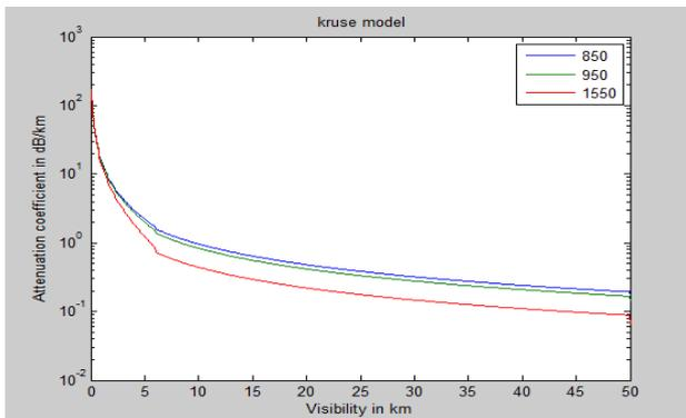
Fig2: Attenuation coefficient versus visibility of Kruse model
