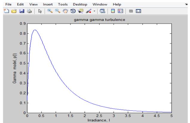
Fig 4: Gamma gamma turbulence model for moderate turbulence
