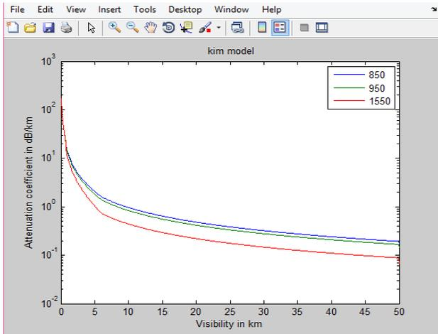
Fig1: Attenuation coefficient vs visibility curve of kim model
