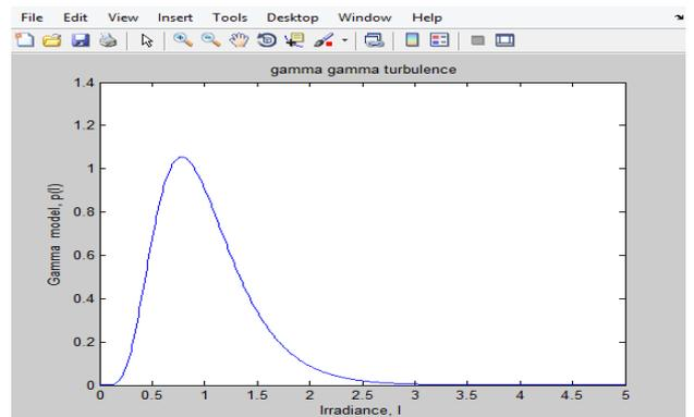
Fig 5: Gamma gamma turbulence model for strong turbulence
